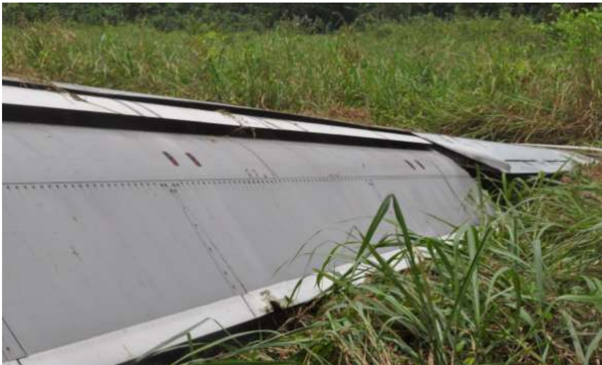
Figure 3: Picture showing damaged right wing
