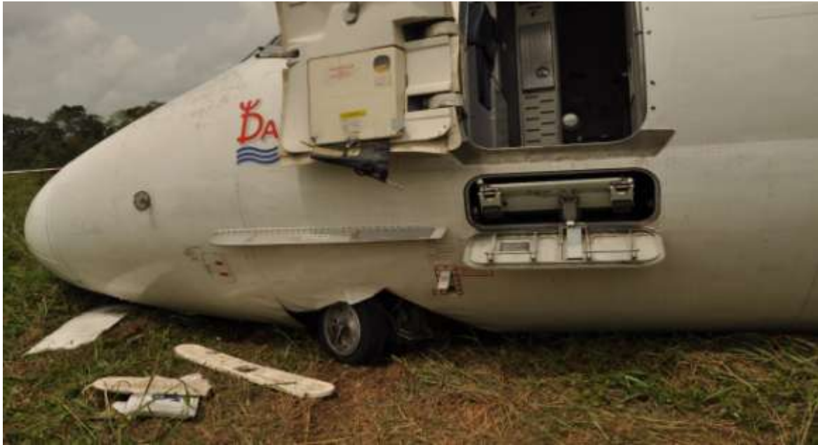
Figure 2: Picture showing the collapsed nose wheel
